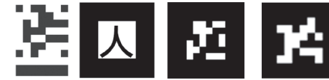
Fig. 2 Examples of the markers from CyberCode 1) , ARToolkit 11) , ARToolkit Plus 14) and ARTag 7) (L to R).
